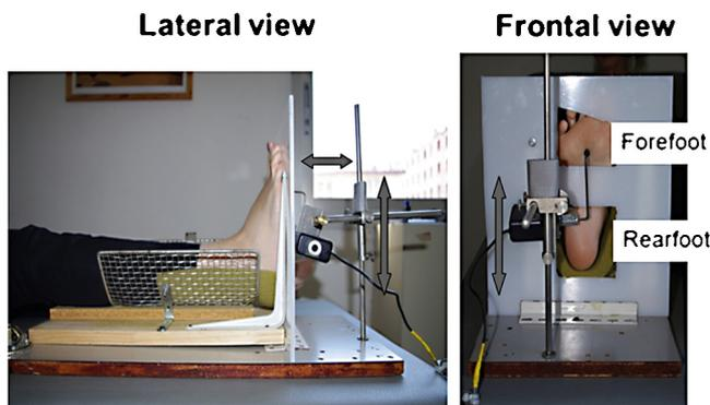
**Fig. 2.** The bespoke apparatus built to apply mechanical stimuli to the forefoot and rearfoot. The mechanical probe is driven by a solenoid and can be moved to apply load to the forefoot or rearfoot as required.
