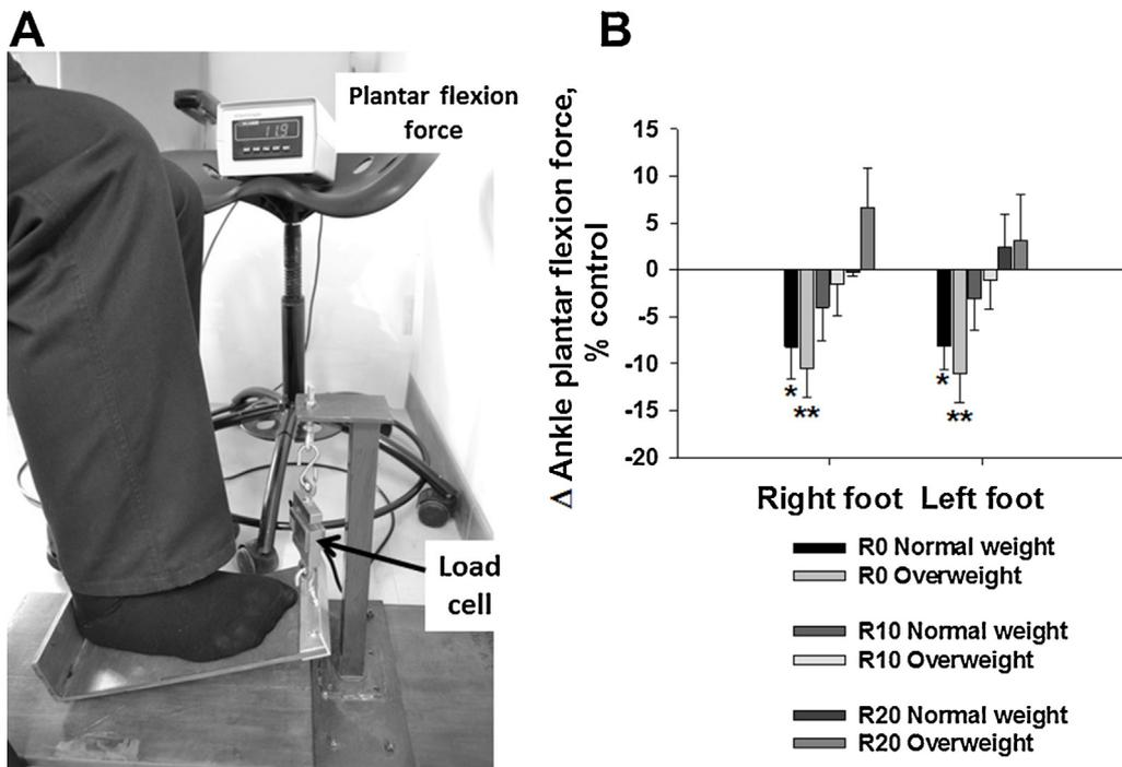
**Fig. 1.** Measurement of the ankle plantar flexion force. (A) The custom-built apparatus used to measure the peak plantar flexion force using a load cell. The subject had no feedback of the produced force. (B) Relative changes in peak ankle plantar flexion force measured after the 6 min walk distance test (6MWT) in both feet of normal and overweight subjects. Asterisks denote significant changes from reference value measured before the 6MWT (\* $p < 0.05$ ; \*\* $p < 0.01$ ).
