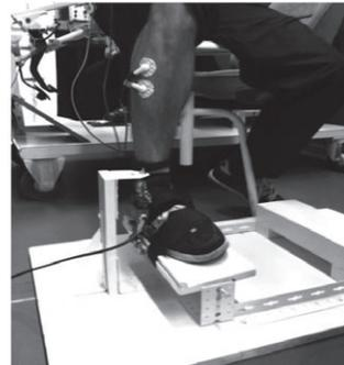
**Figure 1** The driving simulator (a) with details on the surface electrodes positioning (b). The maximal forces produced by the leg extensor and foot inverter muscles were, respectively, measured when the subject was asked to maximally push on the accelerator pedal (b) or to produce inversion movements in the frontal plane (c).
