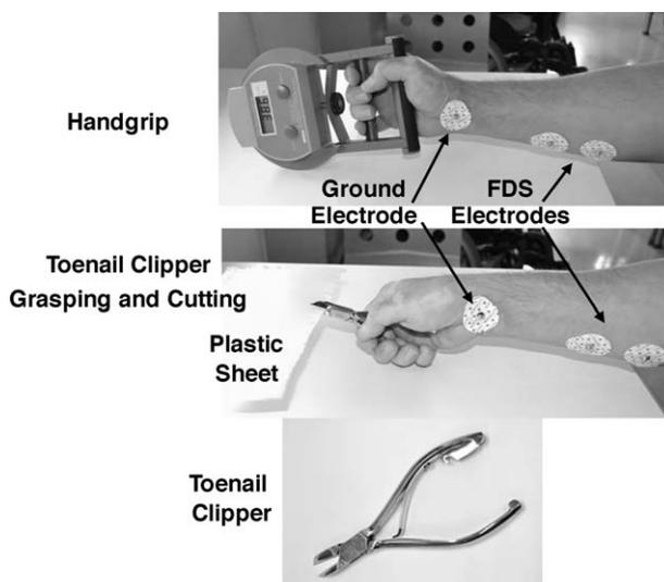
**Figure 1.** Photographs showing the handling positions chosen by the podiatric physician when executing the static handgrip or cutting with the toenail clipper and giving details on the toenail clipper. The positions of the surface electrodes used to record the electromyographic activity from the flexor digitorum superficialis (FDS) muscle are also indicated.
