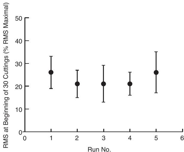
**Figure 2.** Mean  $\pm$  SEM peak values of the root mean square (RMS) of the flexor digitorum superficialis muscle measured at the beginning of each run of 30 successive cuttings with the toenail clipper. The RMS values are expressed as a percentage of the peak RMS values measured in the same individuals executing the maximal handgrip before beginning any cutting run.
